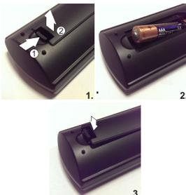
Remove the back cover to reveal the battery compartment and make sure the batteries are inserted the right way round. Suitable battery types for this remote are AAA, IEC R03 1.5V.
